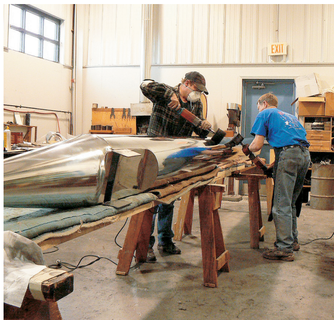
Polishing a facade pipe for Opus 2235
